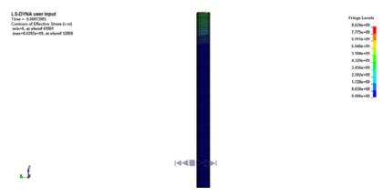
Fig. 8. The stress wave propagation in the drill rod (1)
