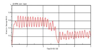
Fig. 12. Bit shock energy and time curve
