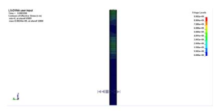
Fig. 9. The Stress wave propagation in the drill rod (2)
